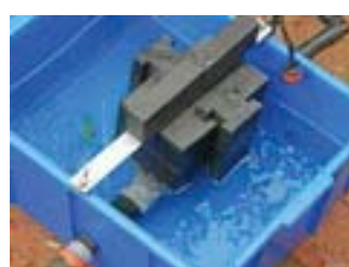
23mm net evaporation between irrigation events (zero gap between magnet and bottom of full slides)
