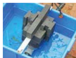
26mm net evaporation between irrigation events (20mm gap between magnet and bottom of full slides)
