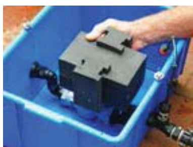
Position the float over the solenoid
