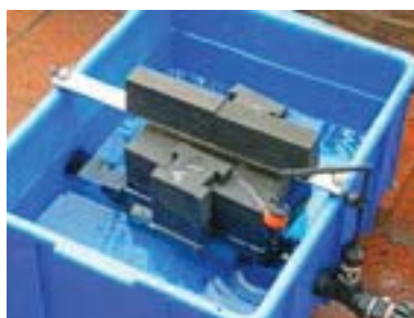
The irrigation starts when the float reaches the low level
