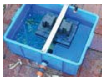
19mm net evaporation between irrigation events (zero gap between magnet and bottom of full slides)
