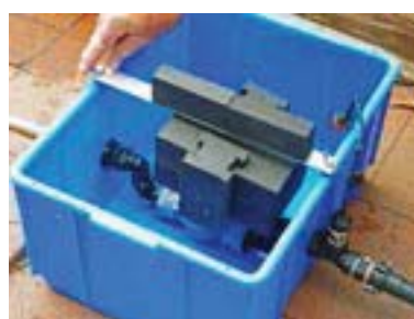
Use the two wing-nuts to secure the aluminium bar
