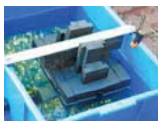
48mm net evaporation between irrigation events (20mm gap between magnet and bottom of cut slides)
