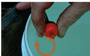
If volume in the measuring container is less than the dripper control volume, turn the control dripper clockwise to reduce the flow rate of the control dripper.
