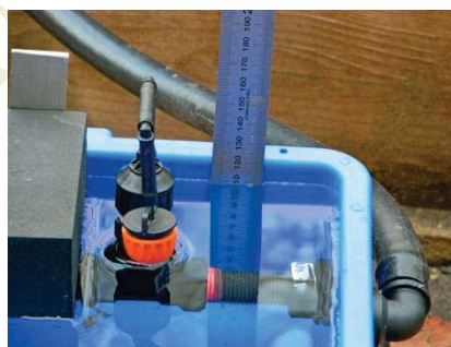
Measure the depth of water in the evaporator at the high level
