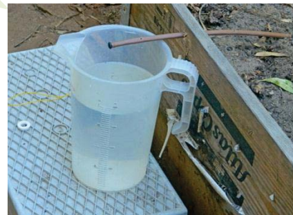
Dripper control volume in the measuring container
