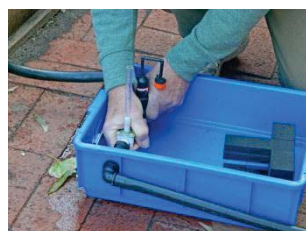
Float shaft must be vertical
