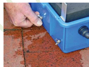
Tighten the wing-nuts
