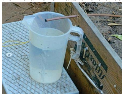
Dripper control volume in the measuring container
