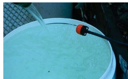
Fill the evaporator with water until the water level reaches the high level
