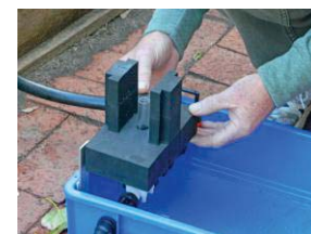
Slide the float over the float shaft
