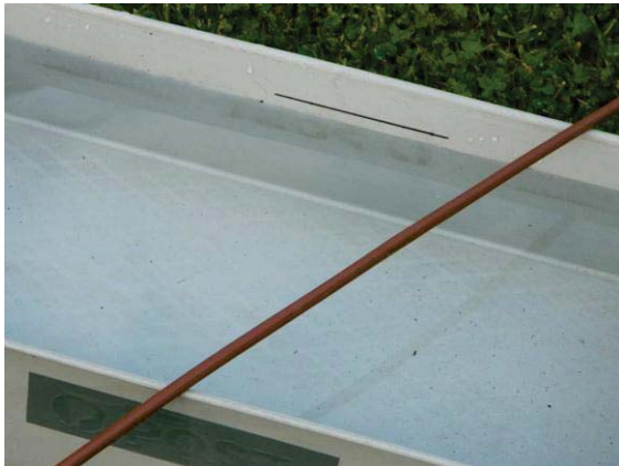
Figure 1. One of the MI drippers drips water into the evaporator during the irrigation event.
