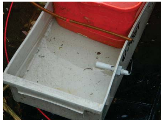
Figure 8. Evaporator for Garden Bed 2 showing the control dripper and a surface area of evaporation of 0.52 m 2 .
