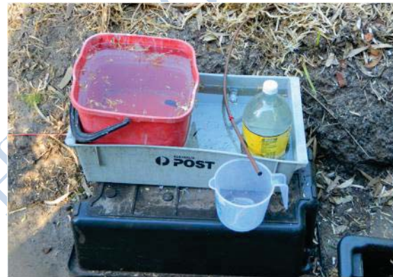
Figure 2. The volume of water emitted by a MI dripper is measured by collecting the emitted water in a measuring cup as shown.
