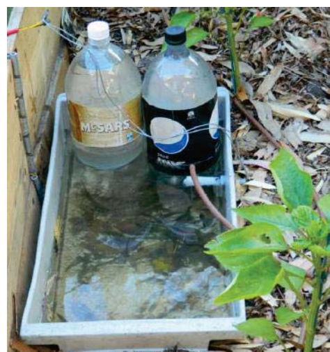
Figure 3. The surface area of evaporation may be reduced by placing full bottles of water in the evaporator.
